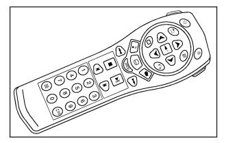
(**Power**): Press this button to turn the RSE screen on and off (also powers up the DVD player if a disc is loaded).
